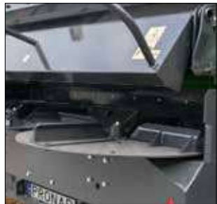
ADJUSTABLE VANES on the spreading discs (N262 AND N262/1) allow the spreading width to be adjusted according to the type of material
