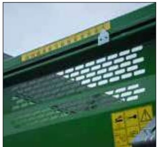
INSPECTION OPENINGS in the front wall of the loading box allow the operator to check the contents of the loading area
