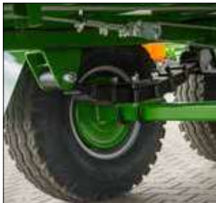
SUSPENSION TANDEM SUSPENSION on Leaf Springs
