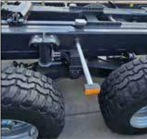
TANDEM SUSPENSION with trailing arms and rigid stub axles equipped with \varnothing 300 \times 135 mm drum brakes (T185)
