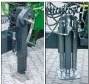
telescopic or hydraulic DRAWBAR SUPPORT LEG facilitates and speeds up machine coupling
