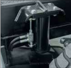
SUSPENSION LOCK HYDRAULIC SYSTEM stiffens the suspension during coupling, loading, unloading and tipping of the container
