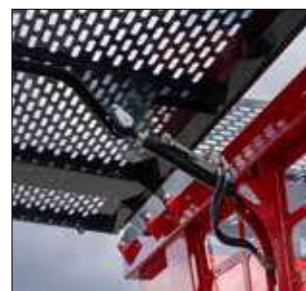
HYDRAULICALLY OPENING FRONT WALL EXTENSION
