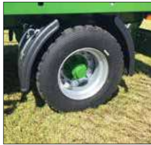
PLASTIC MUDGUARDS mounted in front of or behind the wheel
