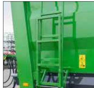
FOLDING LADDER and SIDE WALL STEPS provide safe access to the loading box during operation
