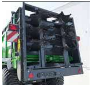
VERTICAL SPREADING BEATER (NV SERIES and N262/2) ensures uniform spreading over a width of up to 12 m
