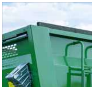
wooden PROTECTIVE STRIP on the upper edge of the loading box protects the upper edge against damage during loading
