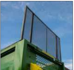
FRONT PROTECTIVE SCREEN protects the tractor cab and windscreen from spreading material
