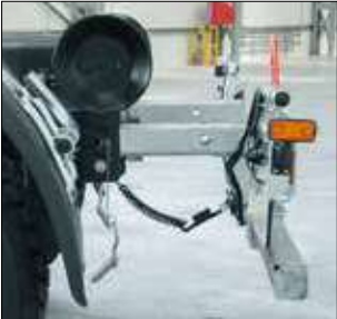
TYPE-APPROVED REAR BUMPER manually extendable and adjustable to several positions, increasing driving safety and allowing the bumper position to be adapted to the length of the transported container
