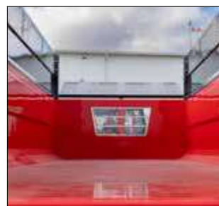
MONOCOQUE LOADING BOX with profiled sidewalls and diagonal reinforcing ribs
