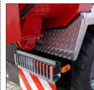
ALUMINIUM MUDGUARD with mud flaps
