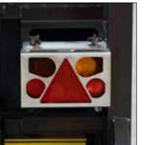
12 V SEALED BULB-TYPE LIGHTS with protective guard
