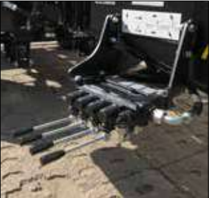
MANUAL CONTROL OF THE TILTING FRAME HYDRAULIC FUNCTIONS
