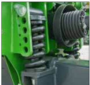
SPRING-SUSPENDED DRAWBAR reduces vibrations transmitted to the tractor
