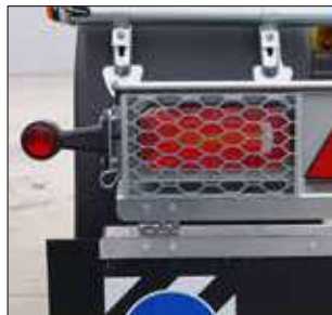
SEALED LED LIGHTS with protective GUARD
