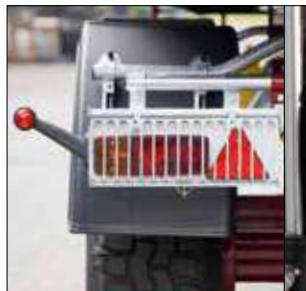
BULB-TYPE LIGHTS with protective GUARD
