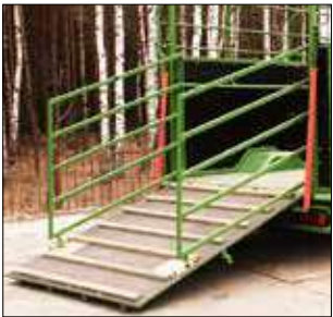
• REAR WALL - RAMP MADE of anti-slip plywood, manually operated, with springs assisting opening and closing
