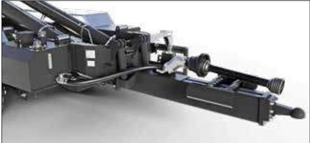
(OPTION T285/1,T286;T286LH) INDEPENDENT HYDRAULIC SYSTEM WITH oil tank, pump, gearbox and PTO shaft , electrically controlled via cable from the tractor cab, operating five vehicle functions (suspension lock, hooklift/tipper mode selection with container locking, hook frame movements, tilting frame movements)
