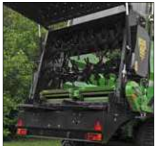
HORIZONTAL SPREADING BEATER with two spreading discs (N262 AND N262/1) ensures uniform spreading over a width of up to 25 m
