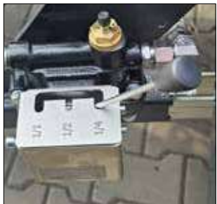
(OPTION T285) MANUAL BRAKING FORCE REGULATOR - hydraulic system
