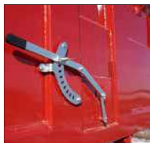
GRAIN CHUTE SLIDE GATE with locking mechanism (OPTION) 3 GRAIN CHUTE SLIDE GATES
