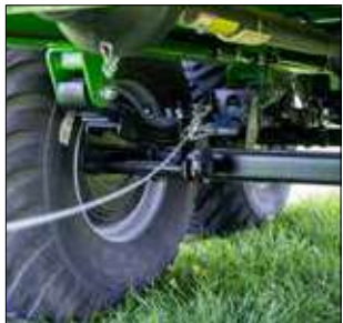
SINGLE-AXLE or TANDEM SUSPENSION with parabolic springs ensures smooth operation even on soft ground
