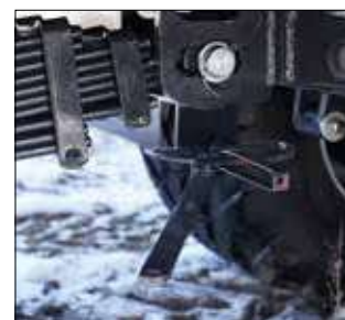
DRAWBAR WITH LEAF SPRING SUSPENSION and PARKING BRAKE
