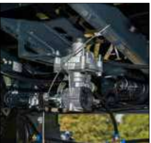
PNEUMATIC BRAKING SYSTEM with automatic braking force regulator (ALB) ensures full vehicle control during transport, even at maximum load
