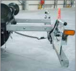
TYPE-APPROVED REAR BUMPER manually extendable and adjustable to several positions, increasing driving safety and allowing the bumper position to be adapted to the length of the transported container
