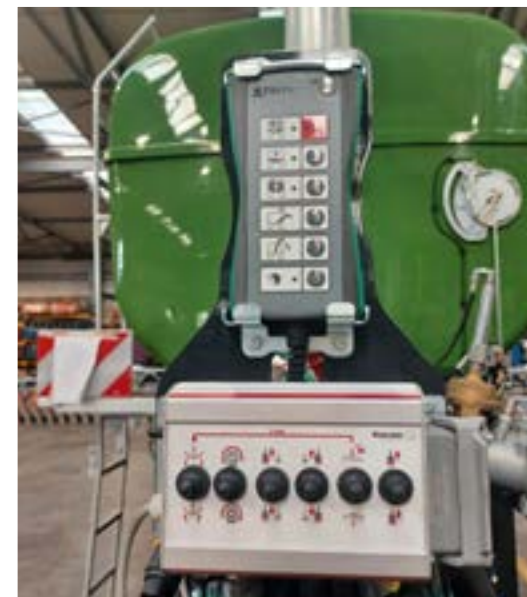
Remote control for slurry tank operations. Steering box for external adapter functions.
