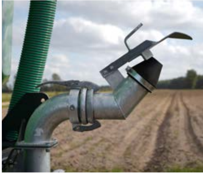
Impact scatterer - Eisele - wave directed downwards, wide spreading even in unfavourable weather conditions (wind).
