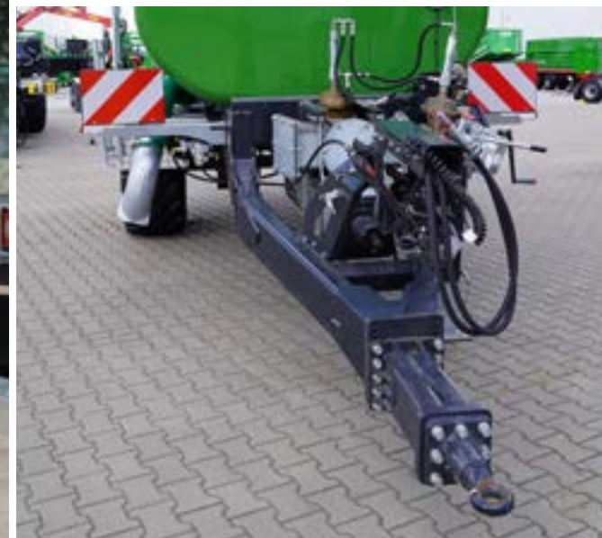
The frame is made of closed profiles Ø250x100x8 mm | Ø9.84"x 3.94"x 0.315" made of high-grade steel.
