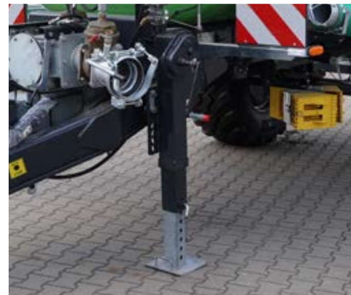
Telescopic support with two-stage gear
