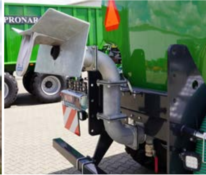
Impact scatterer - Eisele - wave directed downwards, wide spreading even in unfavourable weather conditions (wind).
