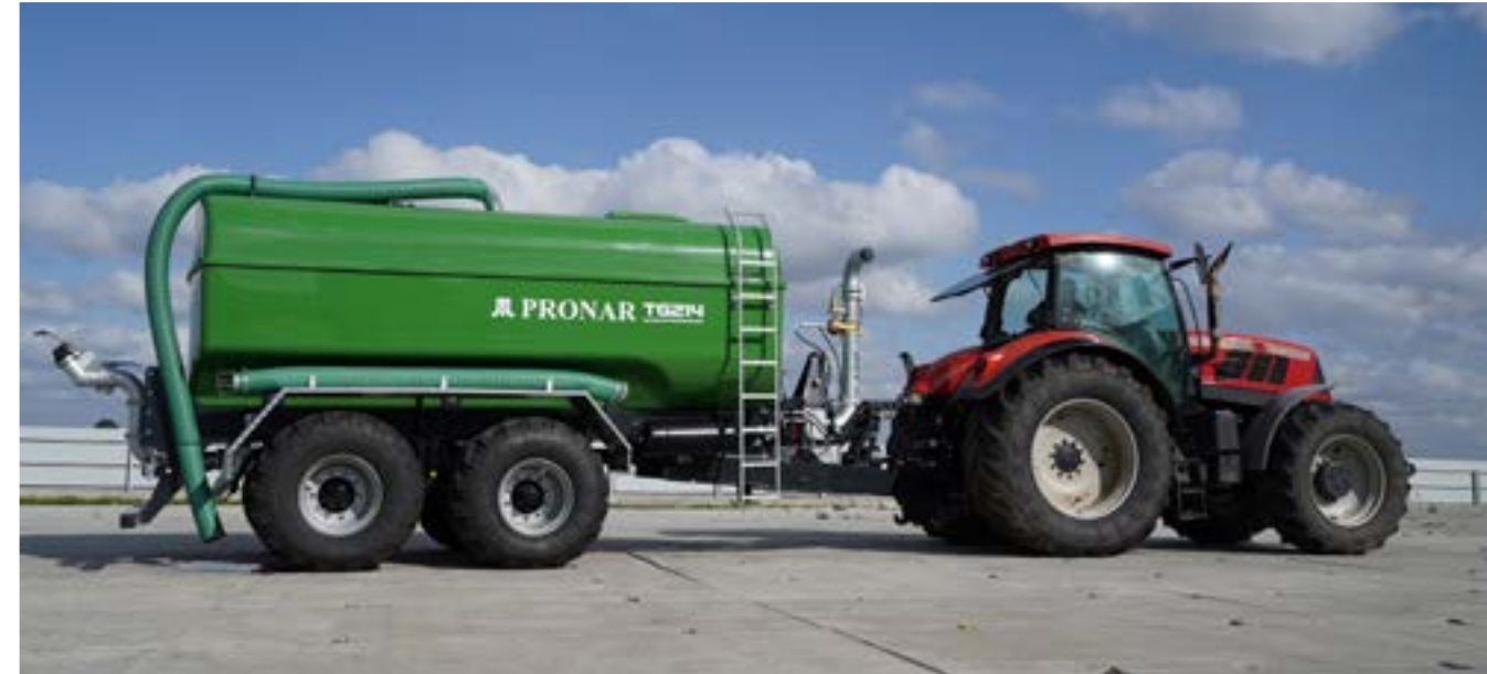
Composite tank reinforced with glass mats ensuring very high chemical resistance - extended machine life cycle. The appropriate thickness of the coating guarantees high durability.
