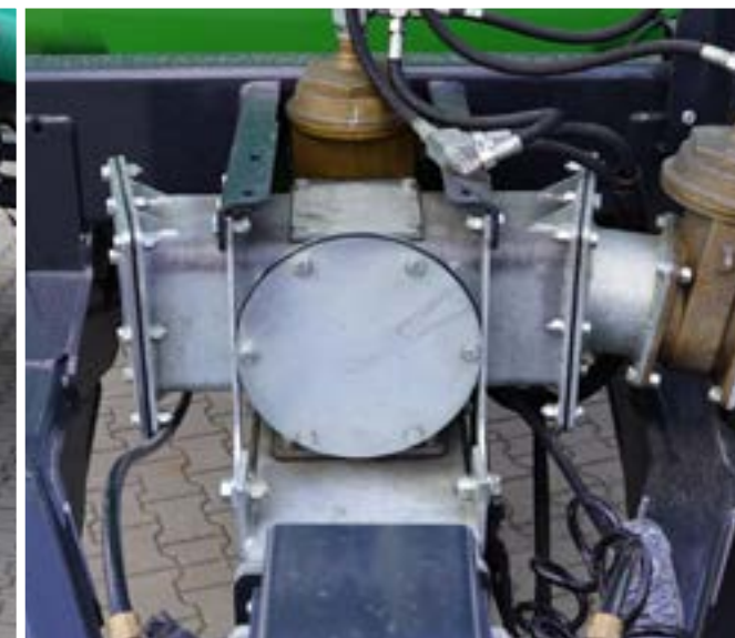
Single-rotor high flow screw pump
