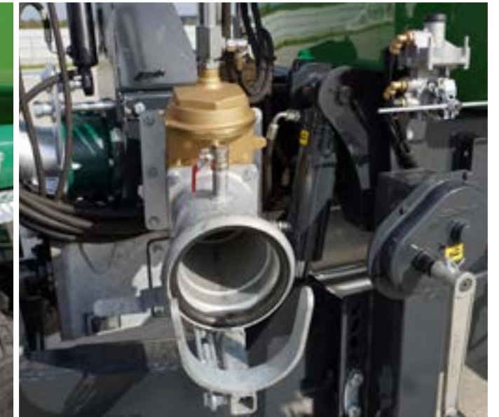
Suction valve 6" | 152.4 mm (Perrot quick couplers and valve with hydraulic cylinder) located on the left side of the vehicle
