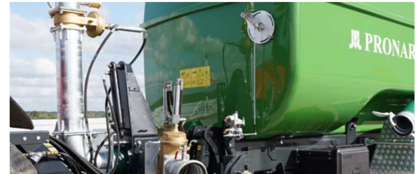
Drum filling level indicator connected to the ALB braking system
