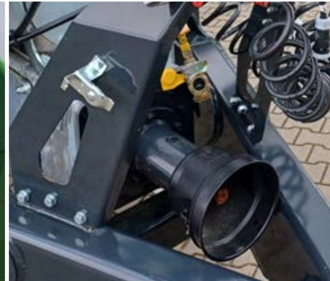
Articulated telescopic shaft for connecting worm pump to tractor's PTO (540 rpm)
