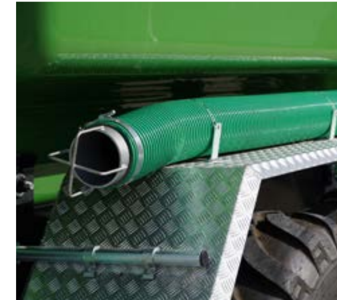
Two 6" | 152.4 mm suction pipes (Perrot quick couplers) 4m | 13,11 ft long. (located on both sides of the vehicle above the fenders)
