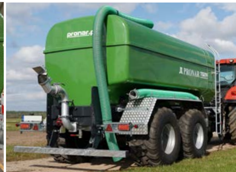
Lower Center of gravity compared to slurry tankers made of steel, which results in higher stability of the tank.
